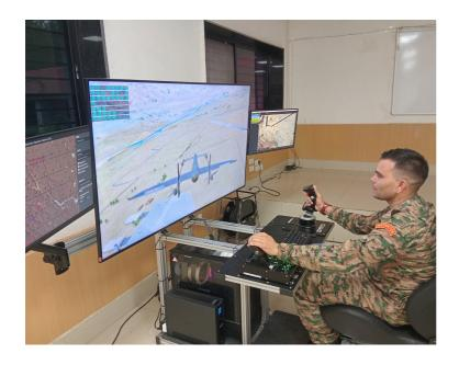
Magister Pro is an advanced UAV flight simulator designed to replicate real-world operations with unmatched accuracy. Featuring a multi-screen setup, powerful computing, and a sophisticated physics engine, it allows operators to experience trueto-life flight dynamics, mission scenarios, and ground control station functionality.
